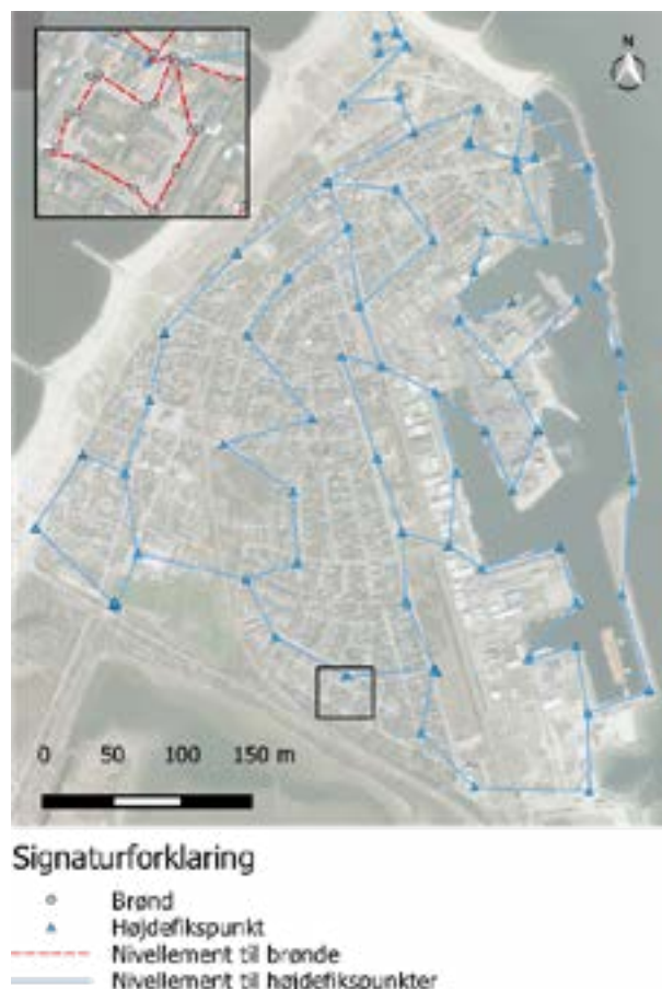
Figure 2. The bench mark measuring campaign in Thyborøn showing how the levelling to each manhole cover is tied to the benchmark network.
