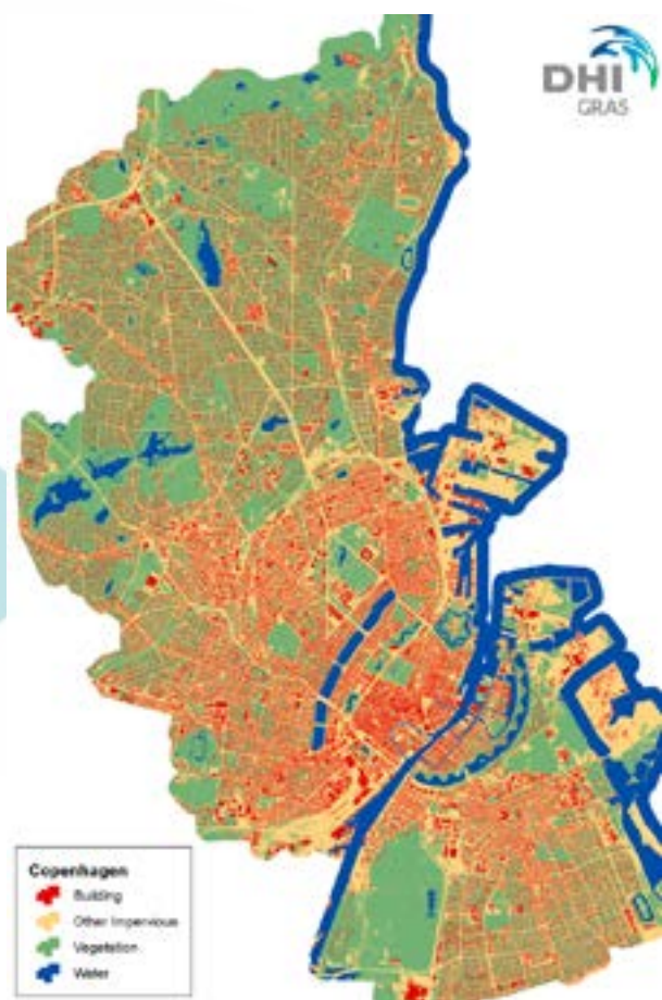
Impervious surface map of Copenhagen, Denmark indicating the coverage of non-permeable surfaces and green areas.
