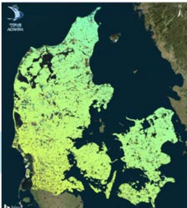
The first nationwide deformation map of Denmark was produced from Sentinel-1 data in 2018 in order to support a wide variety of different uses. The map was updated in 2019 and in 2020.
