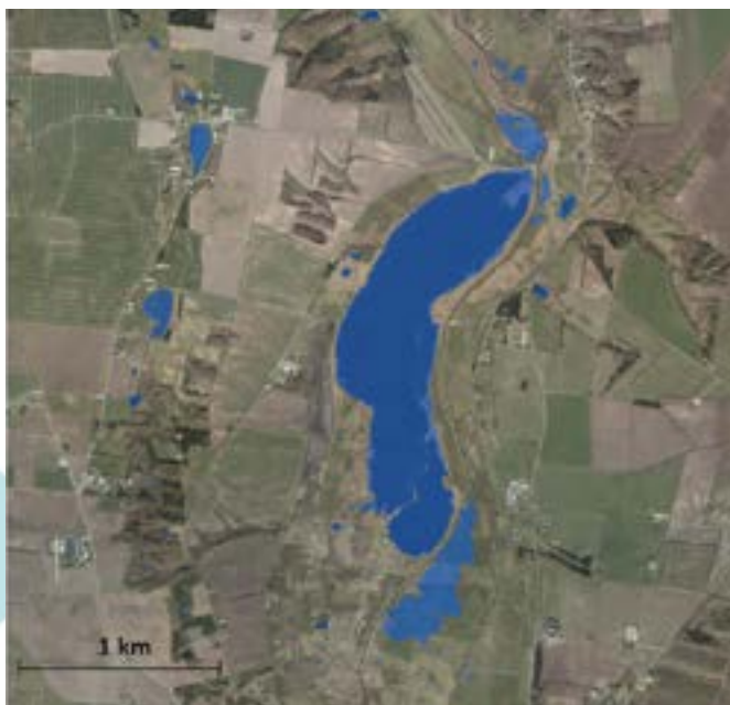
Example of a flood map from the analysis. The blue areas are covered in water and the background is a Danish orthophoto.
